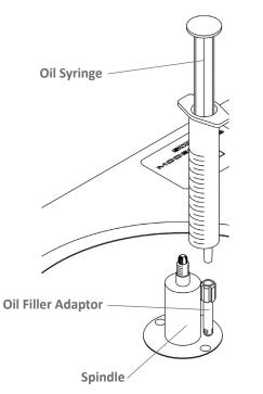
turntable. A measured quantity of oil is provided in the syringe and needs to be injected into the bearing housing.
