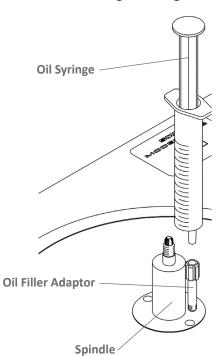
turntable. A measured quantity of oil is provided in the syringe and needs to be injected into the bearing housing.
