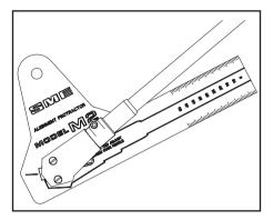
With a record on the turntable, place the alignment protractor onto the record spindle. Check that the VTF has been set to suit the cartridge in use. A small cross indicates the stylus position on the protractor. Move the tonearm out of the armrest and place it so that the stylus enters the indent formed at the centre of the small cross.
