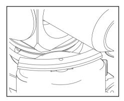
If the tonearm drifts outwards during raising or lowering it indicates contaminant on the rubber pad. To restore positive working, wipe the pad with a damp cloth and repeat with a paper tissue until dry. Clean the underside of the tonearm in the same manner where it contacts the rubber pad.
