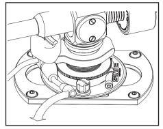
To lower the stylus onto the record move the control lever forwards, in the direction of the arrow, just past top dead centre. This will set the control in motion, at which point it will take over the movement of the lever, giving a smooth controlled descent.
