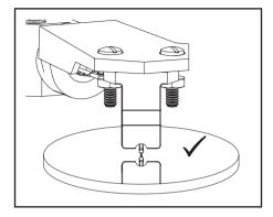
Re-check with the mirror and when satisfied tighten the headshell clamp bolt firmly with the 2mm wrench, avoiding excessive force.
