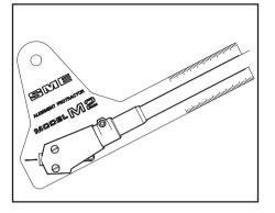
Most cartridges have a stylus- fixing hole dimension of 9.5mm. With these, the outlines of the tonearm and protractor will coincide when viewed directly from above the centreline of the tonearm. With others according to the position of the stylus, it will be necessary to view slightly to the left or right of the centreline; the only requirement for the correct HTA being that the outlines appear to coincide as shown.
