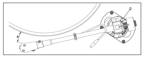
Rotate the pillar to position the armrest conveniently in relation to the turntable. The dimension 'X' should not be more than 75mm or less than 25mm.
