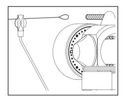
Thread the cord through the guide pulley housing and pass the loop over the anti-skate lever.
