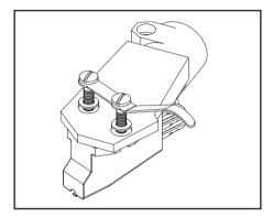
Most cartridges have their own screws. One pair #3-48 UNC x 11mm with nuts and washers are provided.
