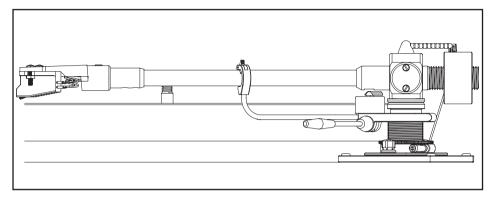
Adjust until the tonearm (with the cartridge fitted) is either level or slightly low at the front end.
