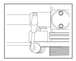
For safety the lever of the lowering control should now be moved into the raised position.
