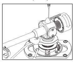
Position the tonearm so that it is clear of the armrest and the cartridge is clear of the turntable. Move the control lever into the lowered position. Balance the tonearm by rotating the weight to move it backwards or forwards as required.
