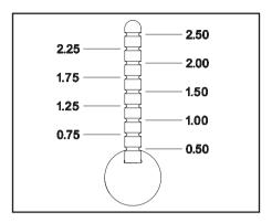
Drop the loop into the groove corresponding to the vertical tracking force being used.
