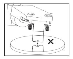
Place a small mirror on the turntable and rest the stylus on it. Viewed in this way any departure from the vertical is accentuated and easily visible.
