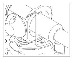
The raising and lowering control is set to suit the majority of cartridges but the height raised above the record can be changed to meet individual needs.
