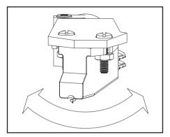
Release the headshell clamp bolt by one quarter turn. The stylus must be clear of the mirror whilst this is done.
