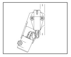
Examine the top of the cartridge. It is important that it presents a good flat face to the underside of the headshell. Before final tightening check that the cartridge is lying parallel to the reference edge of the headshell.
