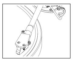
Position the tonearm so that the stylus is over the selected track of the record.
