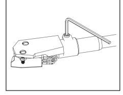
Using the 2mm wrench release the headshell clamp bolt and remove it. The nut remains in its housing in the underside of the headshell where it is retained with adhesive.
