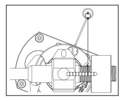
Loosen the inner base clamp nut enough to allow movement of the anti-skate guide. Position the guide so that the cord is approximately 90° to the anti-skate lever when the stylus is over the outer groove of a twelve inch record. Firmly re-lock the base clamp nut. Rotate the guide pulley housing to align it with the cord, which must lie in the groove of the pulley.
