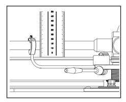
Re-position the alignment protractor about 6mm from the edge of the record. Using the right-hand scale repeat the measurement and compare it with the first one. Adjust with the VTA thumbwheel until similar readings are obtained indicating that the tonearm is level with the surface of the record. Re-lock the pillar clamp screw. View the tonearm in the playing position and re-adjust as necessary.
