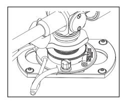
Rotate the control lever fully, in the direction of the arrow, and move the tonearm out from the armrest.
