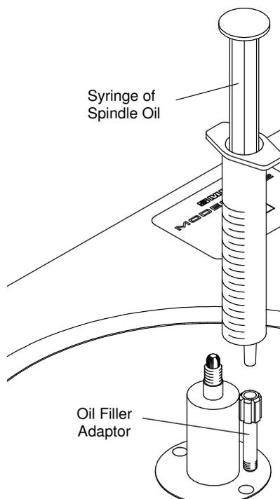
7. Remove the syringe from its packing and insert the tip into the Oil Filler Adaptor, which will be found already fitted to near the spindle. (as illustration left).
